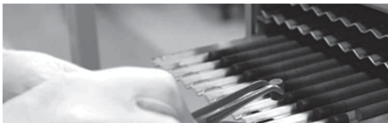
Fig. 19.3 Reactor fuel is in form of ceramic pellets
